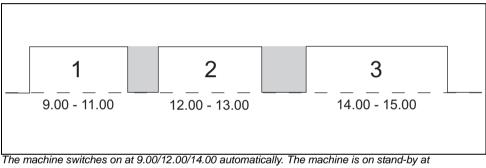
The machine switches on at 9.00/12.00/14.00 automatically. The machine is on stand-by at 11.00/13.00/15.00. During stand-by mode the control panel is switched off and the boiler temperature drops to the set boiler temperature.
