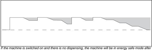
30 min. The temperature of the boiler drops every 30 min. with 5 °C. If there is dispensing after 2 hours the machine is reactivated. The machine uses less energy if there is no dispensing or is left switched on.
